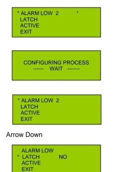
Selecting Enter will allow the operator to change the operation of the relay operation from Non-Latching (NO) to Latching (YES).
