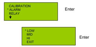
Select the Alarm Relay (LOW, MID, HI) using the down arrow. Once the cursor is on the alarm relay you wish to configure, hold the magnet over Enter. The example LOW will be used. The same operations can be used to set the MID or HI relays.
